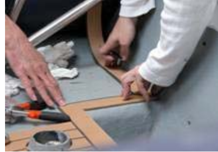
Tape and excess adhesive removed
